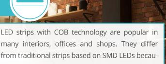
se in COB they create an even line of light without visible points, which is the result of very densely arranged LEDs. An important parameter for COB strips is the colour rendering index, which in this case reaches CRI>90.
